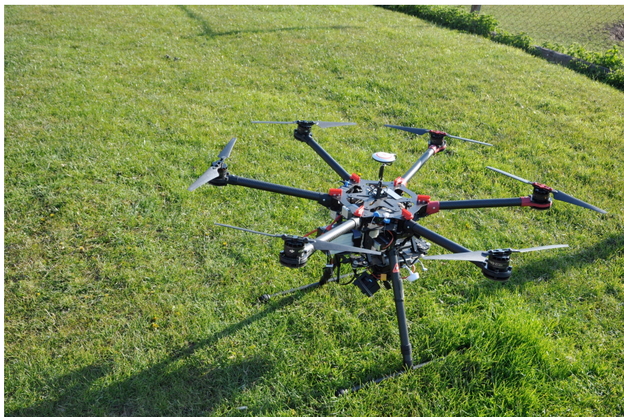
Fig. 2: DJI S900 multi-copter used to obtain preliminary testing data
