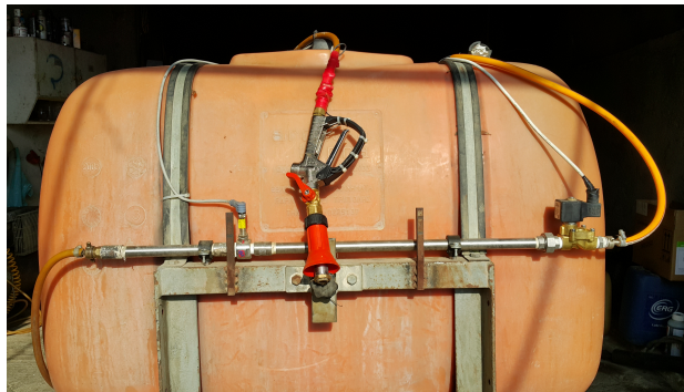
Fig. 3. The developed spraying subsystem installed on a typical small-scale tractor.
