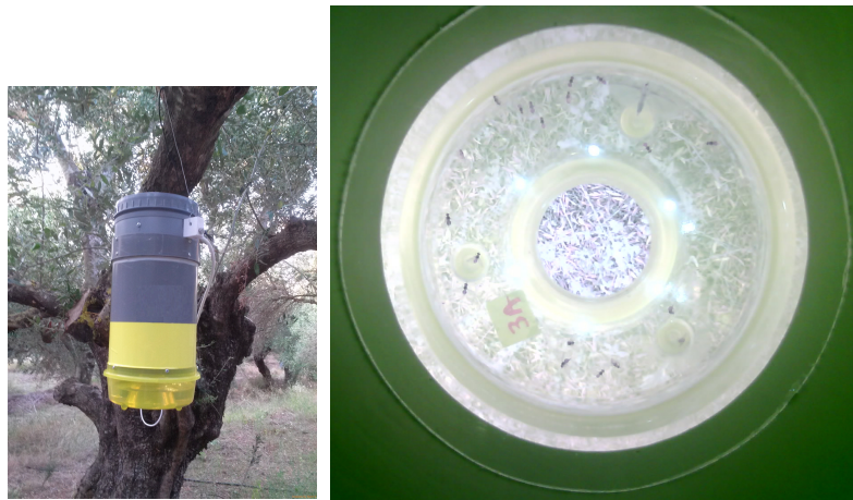
Fig. 2. The “smart” McPhail e-trap installed in the field and a picture of its interior.
