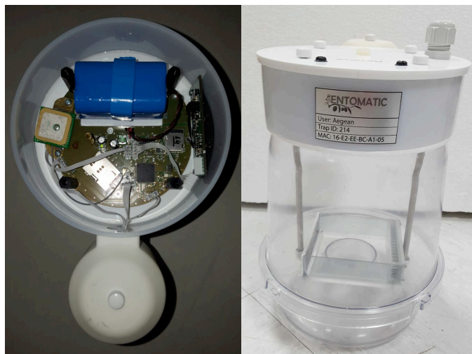
Fig. 2 (LEFT) Embedded electronics. (RIGHT) The electronic McPhail trap.
