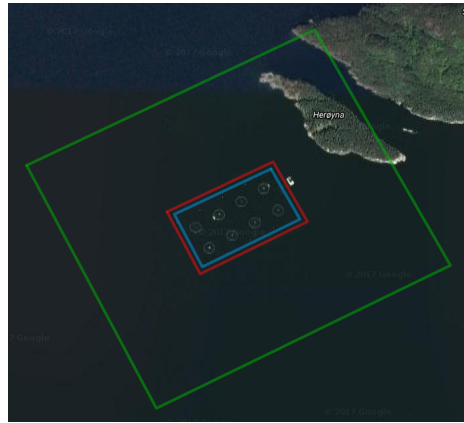
Fig. 1: The Green line show the outer geofence zone, the red line shows the inner geofence zone.
