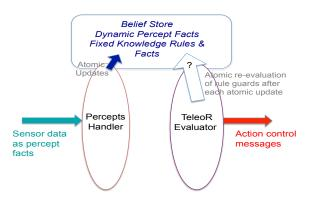
Fig. 1. Simple Two Thread TeleoR Agent Architecture
