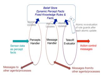
Fig. 2. Single Task Three Thread TeleoR Agent Architecture
