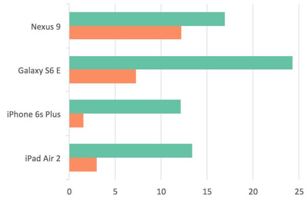
Figure 4: CSV loading times in ms while performing in Unity (green) and D3.js (orange) [lower is better].
