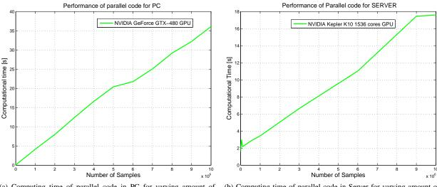
(a) Computing time of parallel code in PC for varying amount of samples
