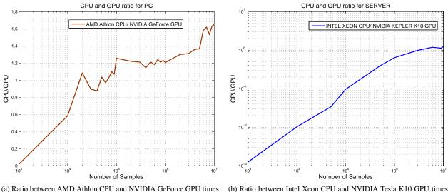
(a) Ratio between AMD Athlon CPU and NVIDIA GeForce GPU times in PC
