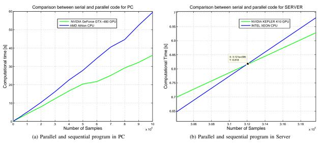
Fig. 4: Comparison between GPU and CPU performance in PC and Server
