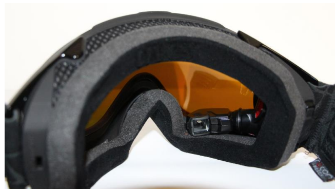
Figure 1. Ski goggle with integrated micro-display
