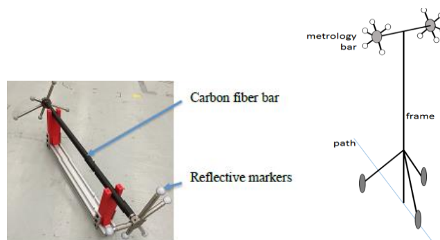
Figure 9. (a) Proposed metrology bar, (b) Example frame used to move the metrology bar.
