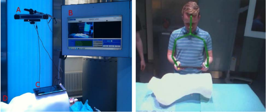
Figure 2: The technical setup of the Magic Lens (left) and an image with person tracking (right).
