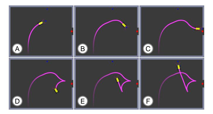
Figure 3: Trajectory of a vehicle as it first approaches a target object (A), manoeuvres the target towards a goal location (B), and then deposits the target at the goal location (C). Following target deposition, the vehicle engages in a reversing behaviour (D) and then begins to move in the direction of a second target (E and F). The progress of the vehicle is indicated by the magenta trail.
