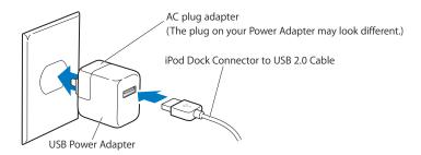
*WARNING:* Make sure the power adapter is fully assembled before plugging it into an electrical outlet.
