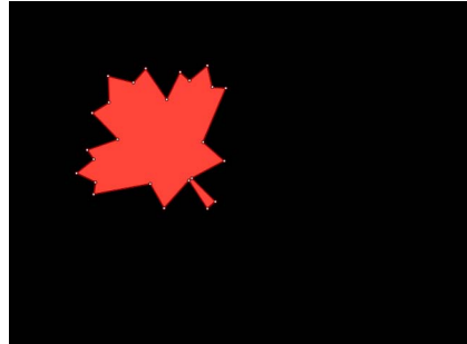
Shape after moving, rotating, and scaling. Note that the control points have also moved.
