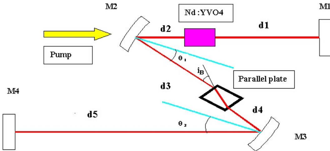
**Fig. 10:** Schematic diagram of a Z-fold cavity of the Nd: YVO<sub>4</sub> laser. The Nd:YVO<sub>4</sub> crystal is the laser gain medium whereas the Brewster plate is used to polarize the light beam.
