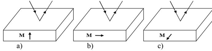
**Fig.8:** The three different configurations of Magneto-Optic Kerr Effects (MOKE) as a function of the orientation of the magnetization  $\mathbf{M}$ ; a) polar, b) longitudinal and c) transverse.
