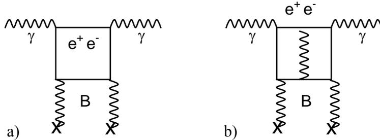
**Fig. 1:** Feynman diagrams for light-by-light scattering producing the magnetic birefringence of the vacuum due to the photon dispersion; a) the dominant term and b) one of the second order diagrams with radiative correction.
