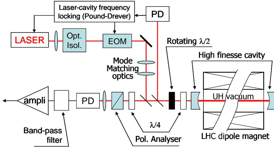
*Fig. 6: Proposed optical scheme for the measurements of the vacuum magnetic birefringence and linear dichroism.*
