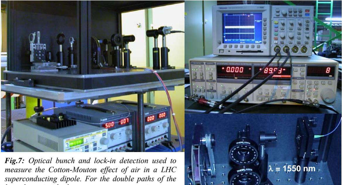
**Fig.7:** Optical bench and lock-in detection used to measure the Cotton-Mouton effect of air in a LHC superconducting dipole. For the double paths of the laser beam inside the magnet aperture, a mirror was positioned outside at one of the magnet extremities.
