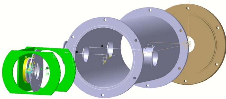
**Fig.3-A1:** Integration of the mirror support inside the end-cap.
