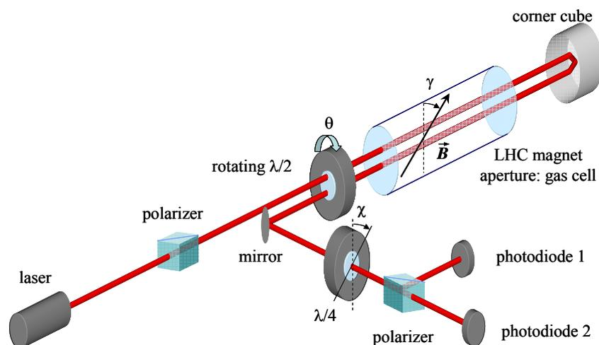
*Fig. 1-A2: Simplified experimental set-up*
