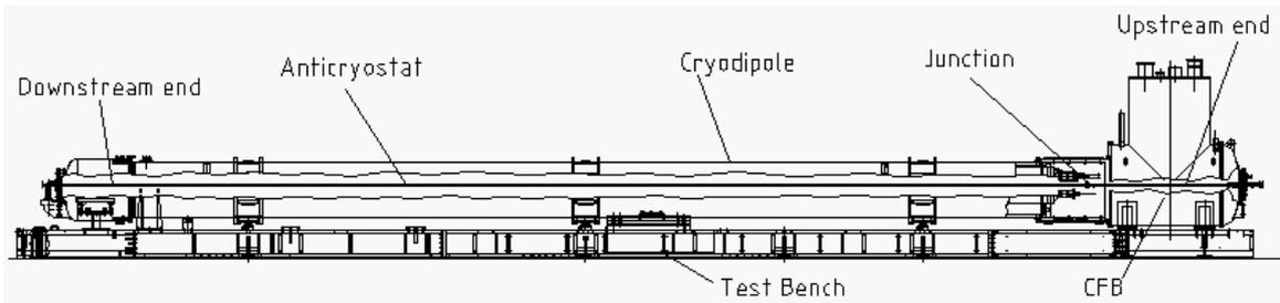
**Fig. 5:** Layout of a cold test bench for dipole magnets equipped with anticryostats and connected to its Cryogenic Feed Box (CFB). The overall length is equal to 19.6 m.
