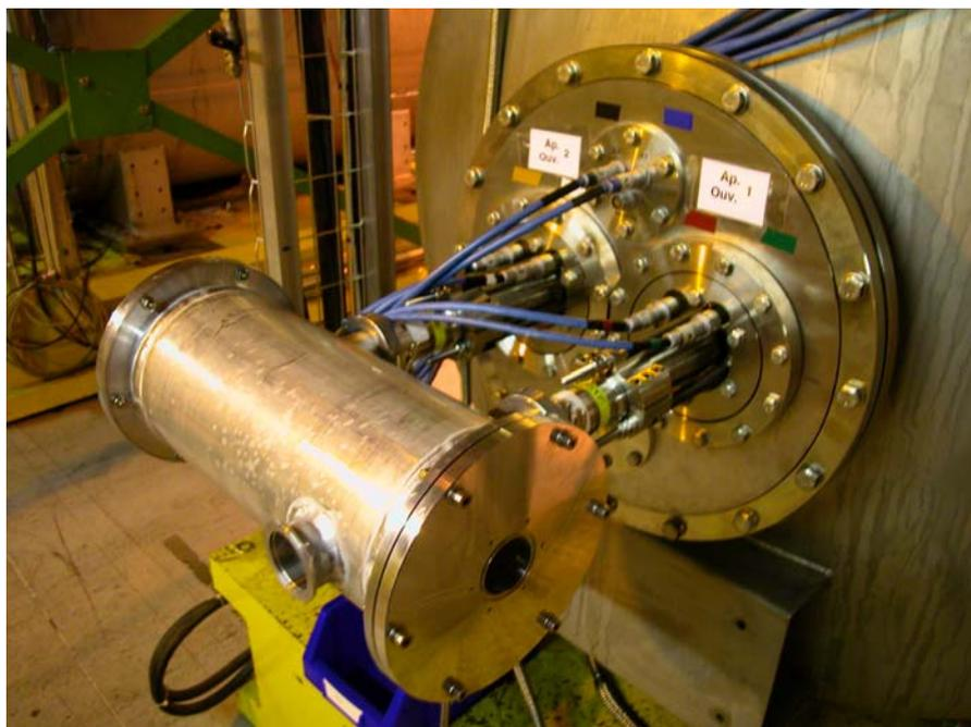
**Fig.2-A1:** Prototype end-caps connected to the Anticyrostats
