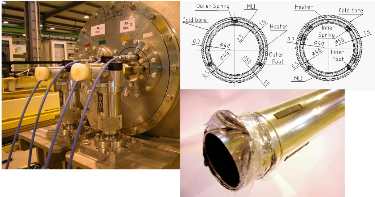
**Fig.1-A1:** Anticyrostats mounted inside a LHC cryodipole
