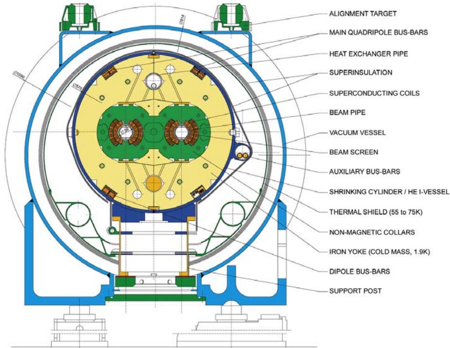
**Fig. 4:** Cross-section of a LHC superconducting main dipole magnet housed inside its cryostat.
