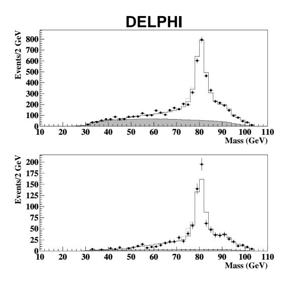
Figure 7: Reconstructed mass distribution in the cscs analysis at 189–209 GeV at preselection (top) and following the complete selection and requiring  $\mathcal{L}$ ; 0.7 (bottom). The expected distribution in the presence of an H<sup>+</sup>H<sup>-</sup> signal, with  $M_{\rm H^{\pm}} = 75 {\rm GeV}/c^2$  and hadronic branching ratio of 100 %, is also shown for comparison (dotted).
