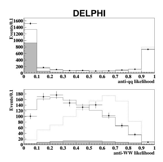
Figure 9: Distributions of the anti-qq and anti-WW likelihoods for the  $cs\tau\nu$  analysis at 189–209 GeV. The anti-qq likelihood is plotted after applying all other cuts and the anti-WW likelihood at the final level. Data and SM background are indicated as in figure 8. The expected distribution for a 75 GeV/ $c^2$  charged Higgs boson signal is shown as a dotted histogram with arbitrary normalisation.
