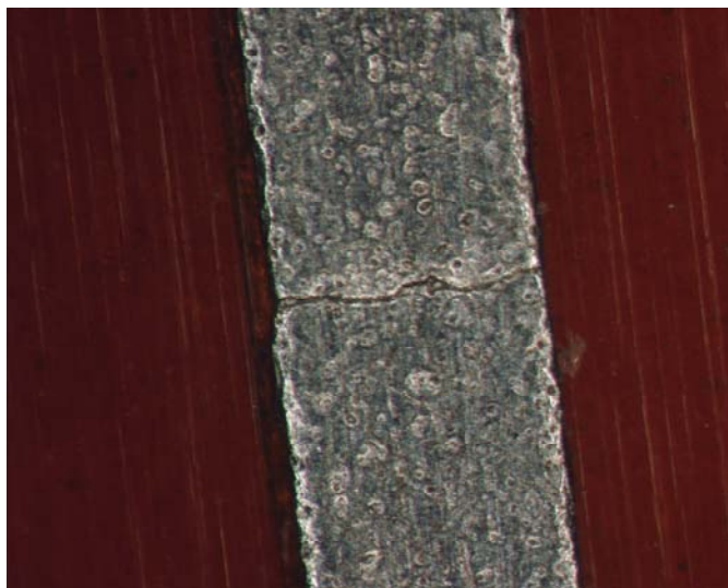
Figure 29. Crack on an HV line of an Al/kapton LMT.
