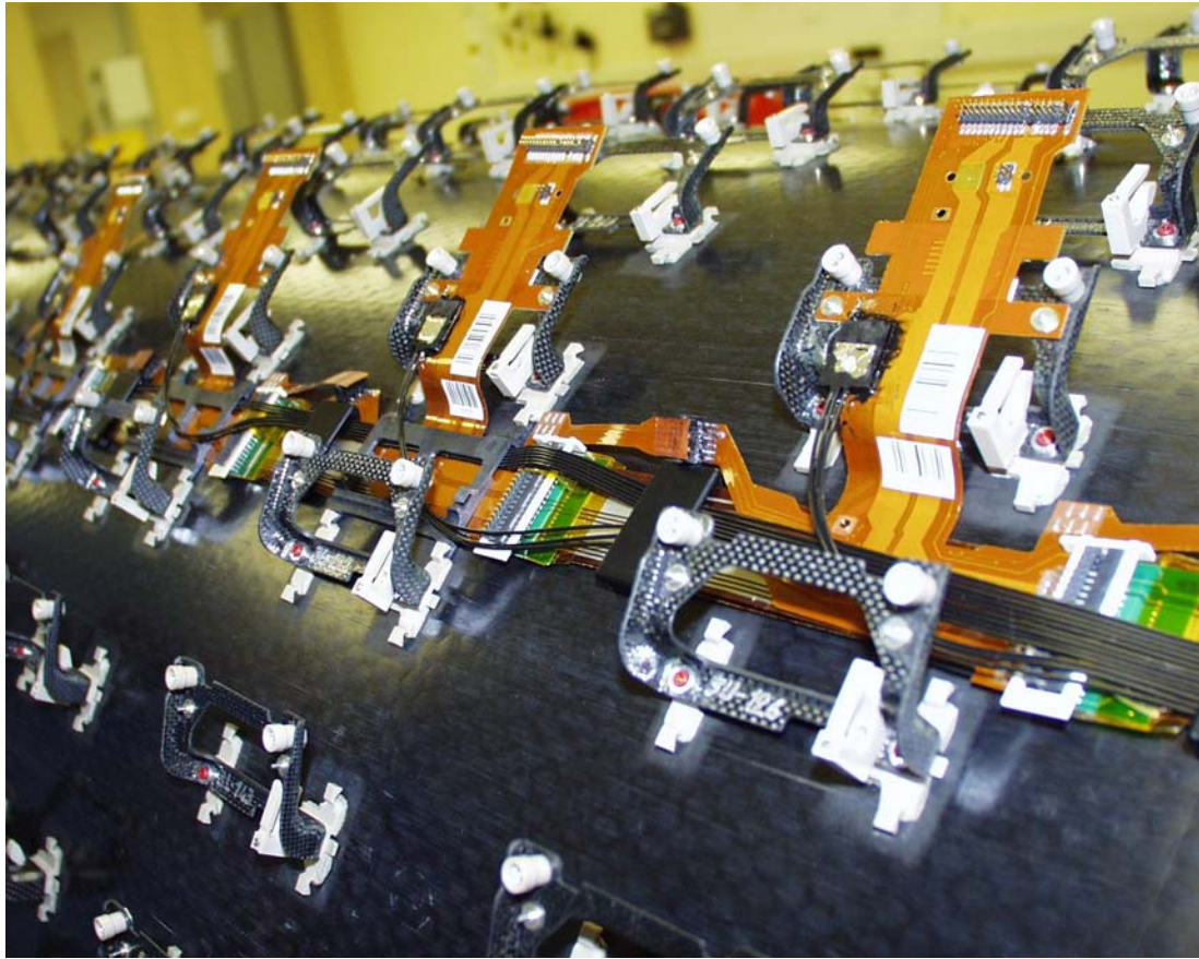
Figure 12. Photograph of part of a barrel harness after mounting onto a barrel. Four opto-flex circuits (out of six on the harness) and the associated fibres are visible.
