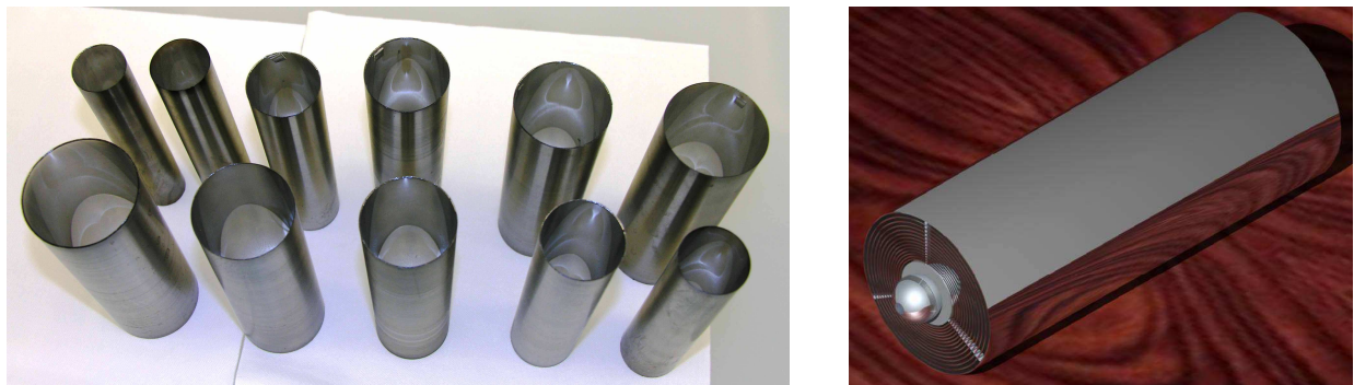
Figure 23: Left: Photograph of 11 iridium coated polycarbonate substrates, prior to integration into the optic assembly. Right: Engineering drawing of the completed nested optic.
