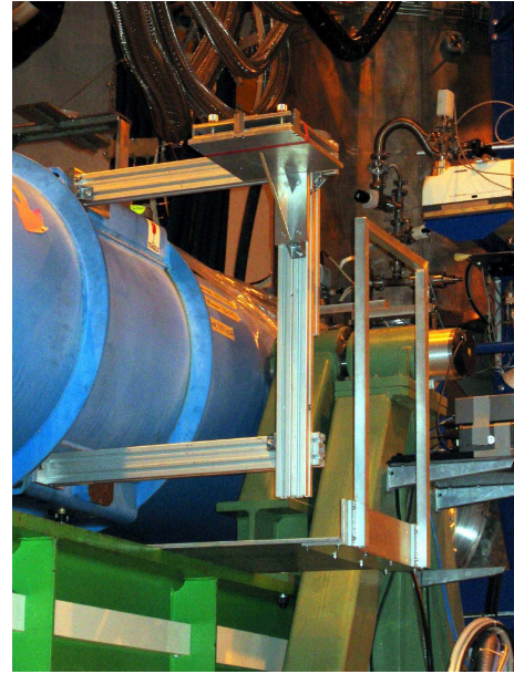
Figure 16: Left: The filming system is mounted on a tiltable platform on the console fixed to the Rexroth Profiles. It simplifies the vertical alignment of the optics. A support allowing movements of the camera in all spatial directions holds the ST-7 and is screwed to the inclinable platform. Right: The new side arm for the filming system constructed by using Rexroth Modular Profile Systems is fixed to the magnet. A console is attached to the vertical profile. It can be moved up and down to bring it into any desired position. Thus a rough adjustment of the filming system can be performed.
