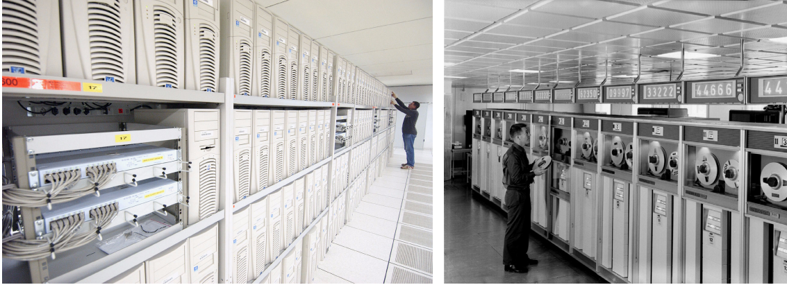
Figure 2-14 Today's PC farm in the new computing centre (left). The tape unit reel display system (RDS) in 1965 (right).
