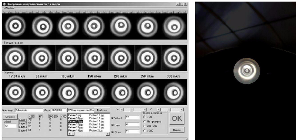
Figure 5-5 Straw straightness is inspected with the help of concentricity of the light pattern. At production site it is done with a CCD camera. The window on the left shows the correlation of the change of light pattern with increasing lack of straw tube concentricity. For the gas-monitor assembly, a visual check against a light source is sufficient (right).
