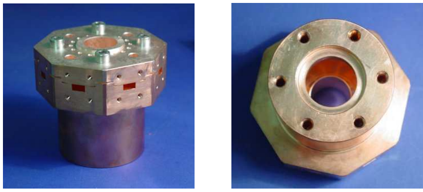
Figure 22: Low RF power prototype of the PETS Power extractor
