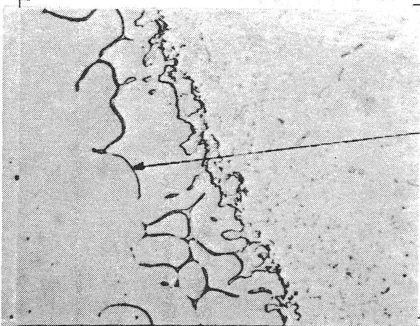
Metallographic section showing copper diffusion in the stainless steel grain boundaries.
