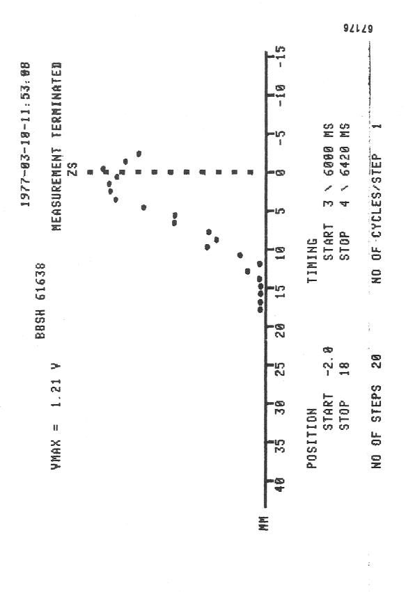
Fig. 5 Density distribtuion at the electrostatic septum ZS for a 7 ms spill at QH = 27.
