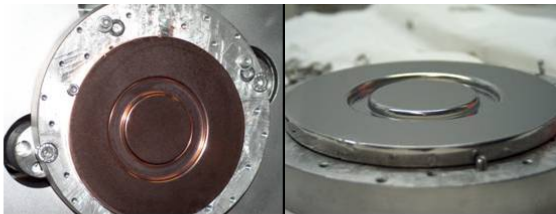
Fig.2a. Large Cu sample on its holder before deposition.
