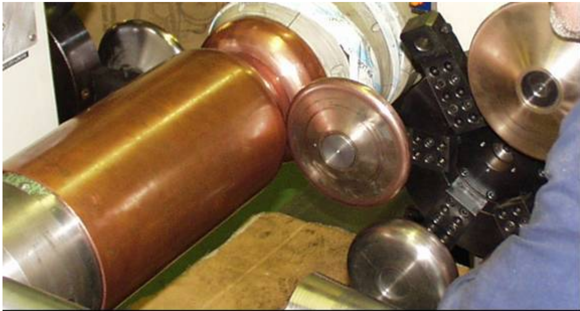
Fig. 3: Phase of the double turret necking process during the spinning parameter definition action.
