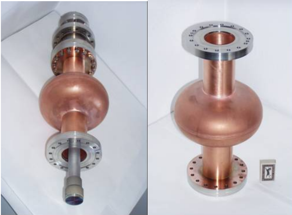
Fig.2. TESLA-type copper cavity equipped with vacuum flanges needed for installation at the UHV-arc stand.
