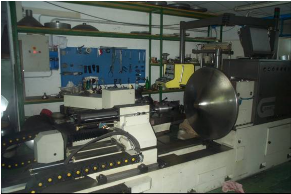
Fig. 1: The spinning lathe used for the fabrication of seamless cavity prototypes. The lathe has only one turret which hold the rollers.
