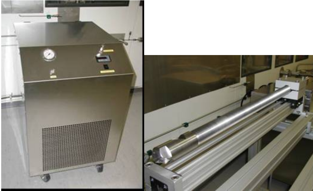
Fig. New CO 2 - cooler/purifier unit (left) and horizontal spraying cane assembled on the linear drive (right)
