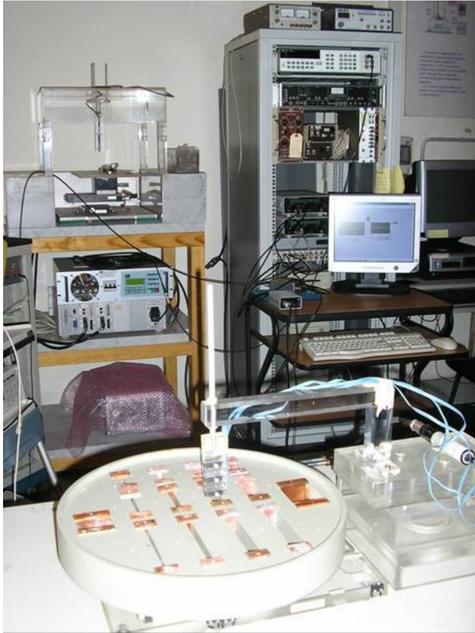
Fig. 2 The scanning flux gate apparatus.
