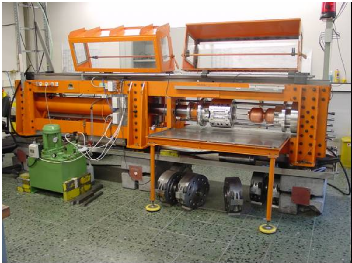
Fig. 4: View of the hydroforming machine
