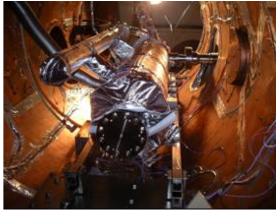
Figure 1: 9-cell cavity set up in CryHoLab and high power coupler connected.
