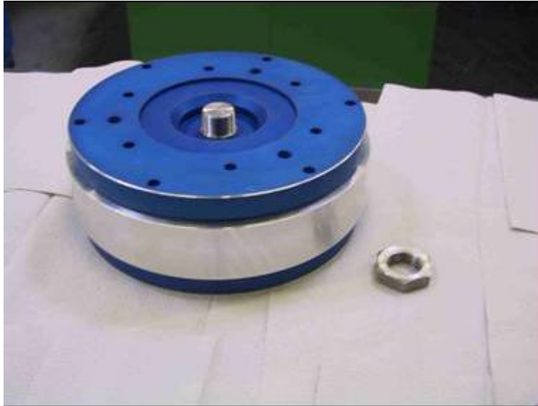
Figure 1: Complete Fixture for end half cells with both caps
