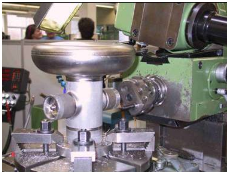
Figure 4: Preparation for welding gun coupler flanges on a milling machine
