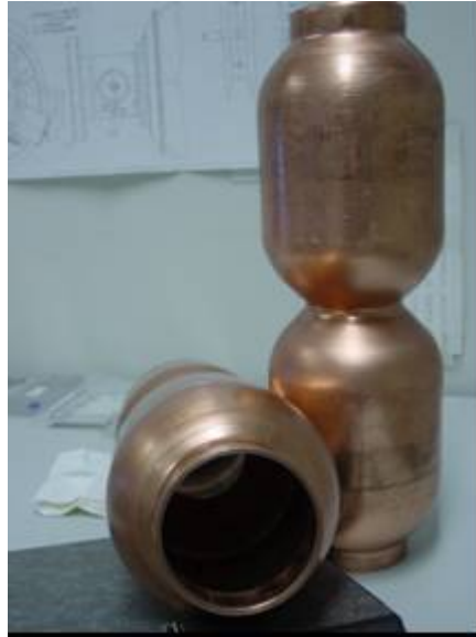
Fig. 3: Necking at the tube end and tube middle implemented by necking machine
