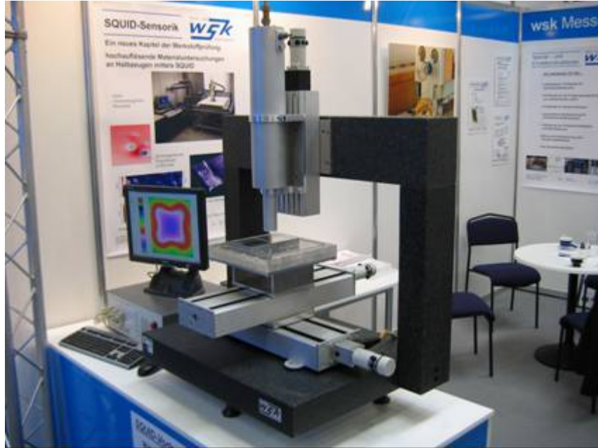
Fig. 1: View of a SQUID scanner for Nb sheets
