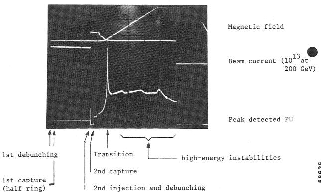
Note that the capture efficiency is about 90%. Untrapped particles correspond to the abrupt beam loss at the beginning of the parabola.
