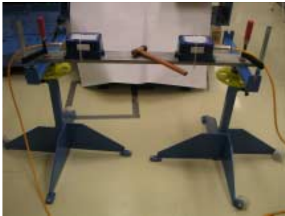
Figure 1 : Photo of the initial sensor set-up for the hammer test.
