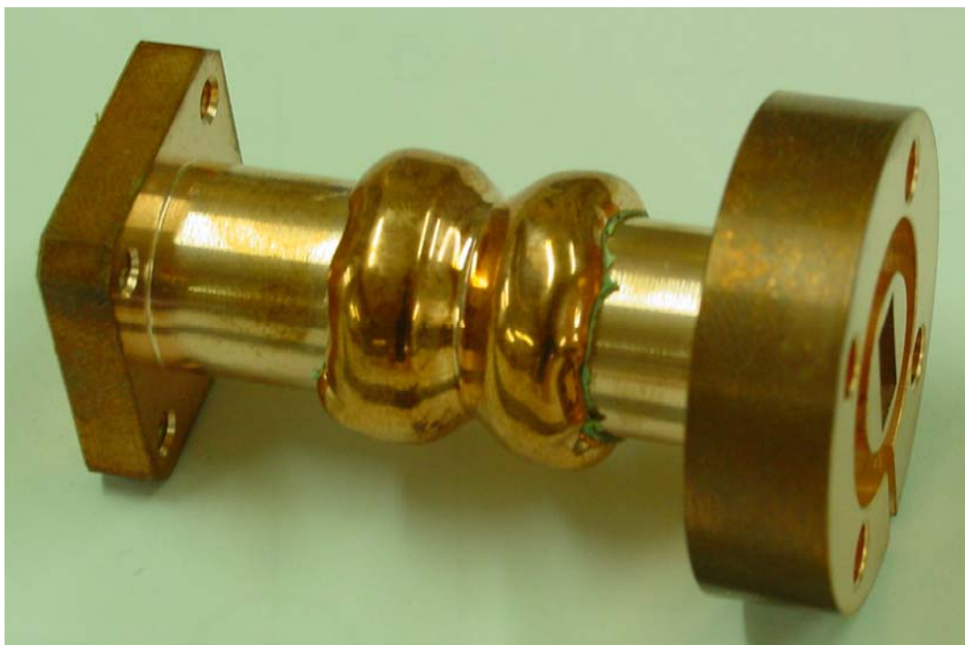
FIGURE 17. Cu-plated rf window before (a) and after (b) Cu-deposition.
