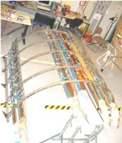
Figure 4: Cable trays inserted into squirrel cage, which goes over the TRT End-Cap wheels.
