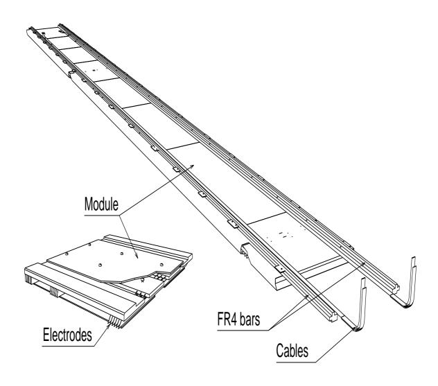
Figure 1: Perspective view of a presampler sector.
