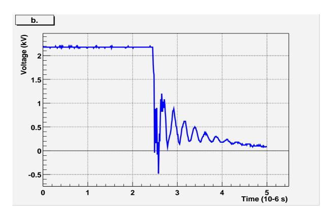
Figure 5: Voltage measurement on the module HV lines during discharge. The voltage drop at 0.8 s and 2.5  $\mu s$  respectively are due to the 1 M $\Omega$  resistor being bypassed by an electrical arc.
