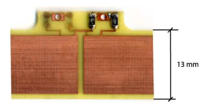
Figure 2: Photograph of the central part of an anode (see text).
