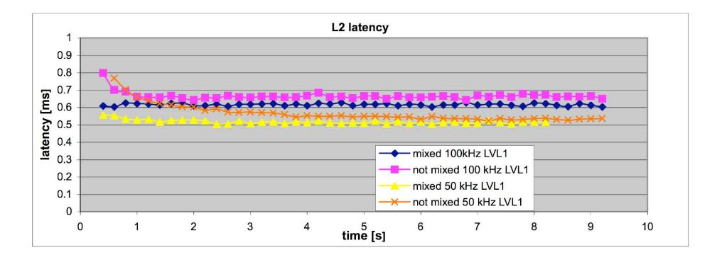
"Not mixed": LVL2 traffic and EB traffic via different switches and via different ROS network interfaces
