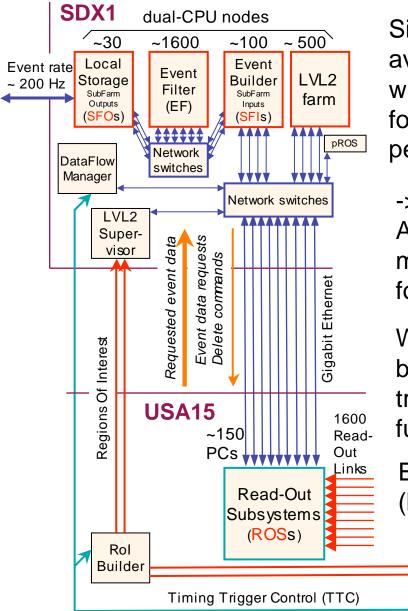
Simple model ("paper model") used to predict average number of ROS PCs and ROLs from which data is needed for LVL2 trigger processing, for example for design luminosity trigger menu, per first-level accept: **16.2 ROLs or 8.4 ROS PCs**
