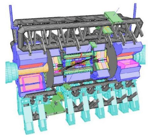
ATLAS is a multi-purpose detector for the LHC collider ( $E_{CM}$ =14 TeV)
