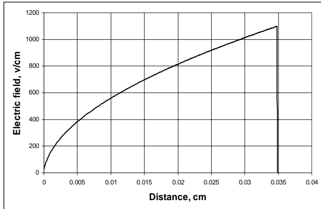
Fig. 3. Electric field distribution calculated for CID with hole injection at: J_{inj} = 1 \cdot 10^{-5} \text{ A/cm}^2 , V = 30 \text{ V} , N_{dl} = 2.8 \cdot 10^{12} \text{ cm}^{-3}
