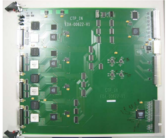
Figure 5: Photograph of the CTP_IN module
