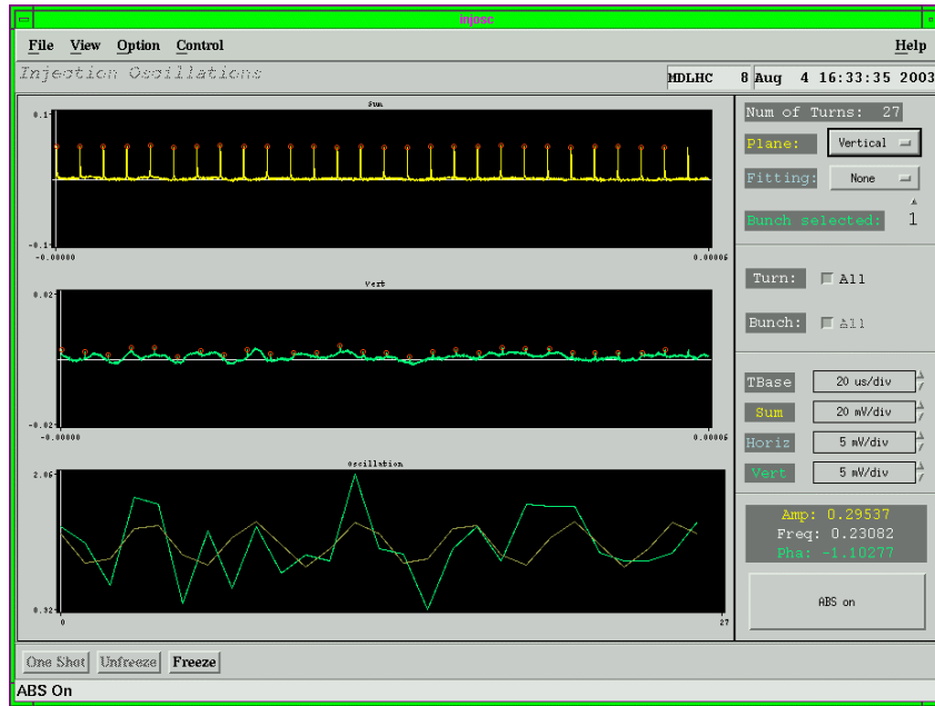
Figure 3.7: Correction of the vertical coherent oscillations at PS injection.
