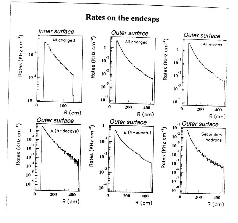
Figure 27: Muon rates on the endcaps.
