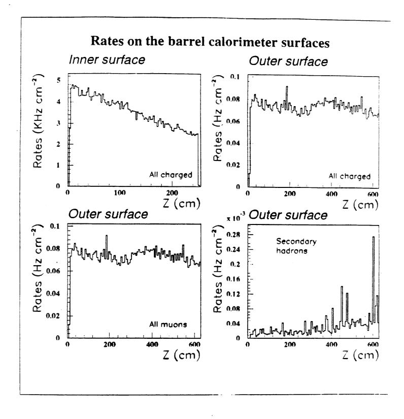
Figure 26: Muon rates on the barrel calorimeter surfaces.
