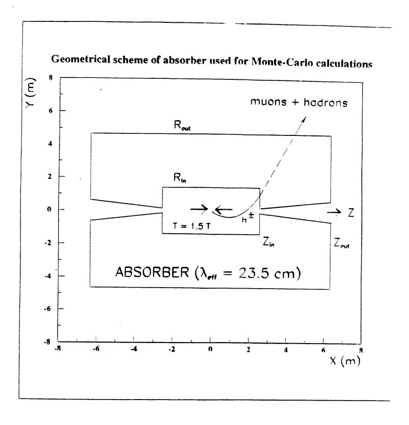
Figure 8: Scheme of geometrical calculation in the fast Monte - Carlo program.
