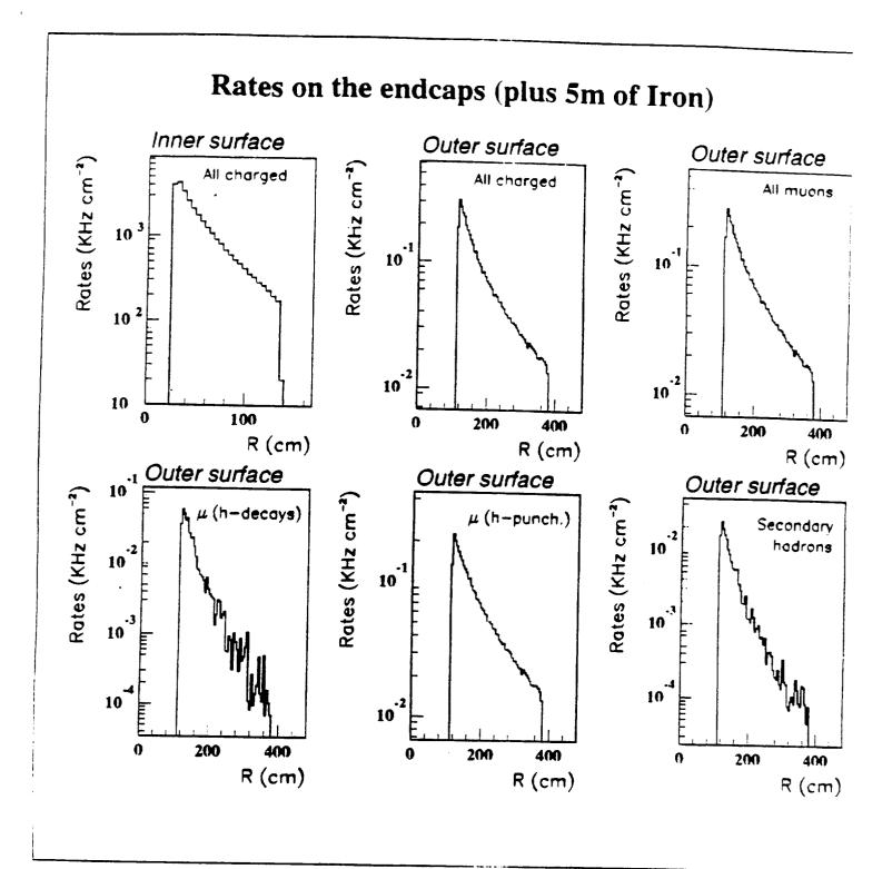
Figure 28: Muon rates on endcaps with additional 5m of iron absorber.
