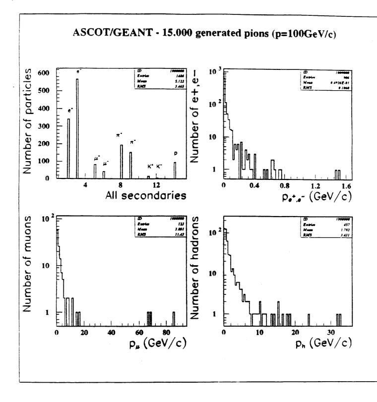
Figure 4: Secondary particles of the hadron showers leakage induced by pions being generated with  $100 \ GeV/c$  initial momentum.
