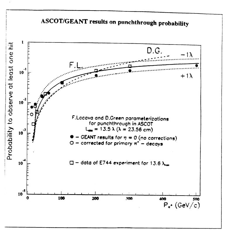
Figure 2: Probability to observe any hit in ASCOT muon system (GEANT calculations) in comparison with Lacava parameterization.
