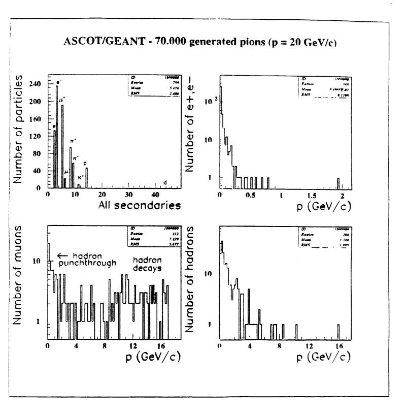
Figure 3: Results of GEANT simulation for secondary particles in first muon chamber. The particles were emitted during the development of the showers caused by single pions with initial momentum  $20 \, GeV/c$ .
