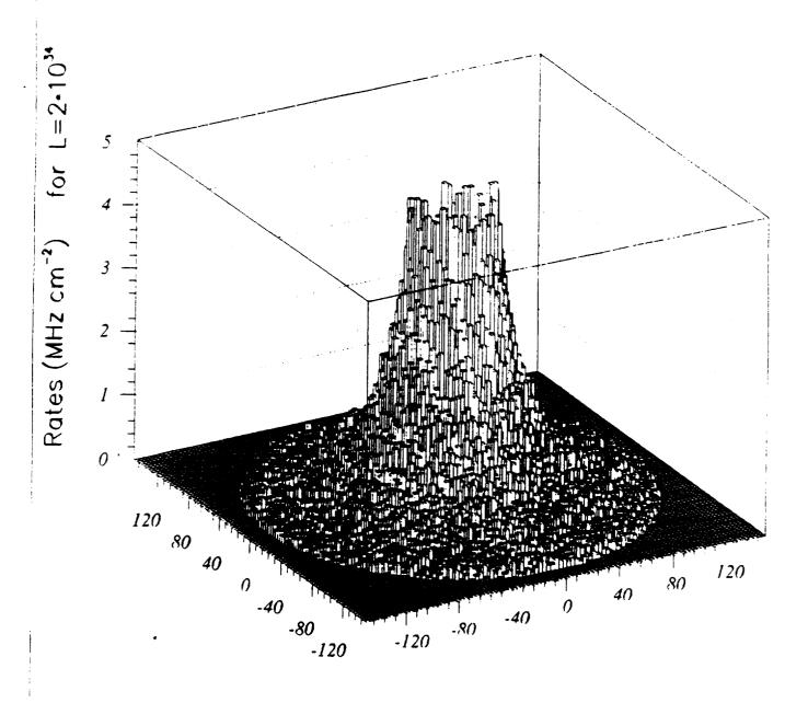
Figure 24: Rates charged secondary particles on the inner surface of endcap calorimeter.
