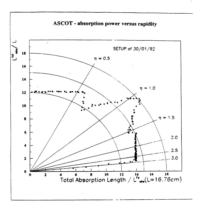
Figure 31: Total apsorption thickness of combined electromagnetic and hadron calorimeters and tail catcher for different rapidities (ASCOT Setup of 30/01/92).
