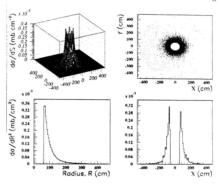
Figure 23: Different projections of the cross section of muons and secondary particles from shower leakage on the outer surface of endcap calorimeter.
