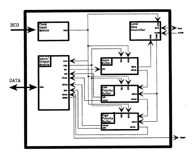
Figure 3 A functional layout of the Bus Handler (BH).
