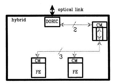
Figure 1 A schematic layout for a hybrid showing the serial bus between the CM part in the Front End chips and the CM chip.
