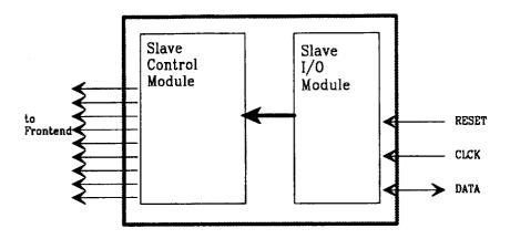
Figure 4 A schematic layout of a controlling slave module.
