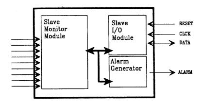
Figure 5 A schematic layout of a monitoring slave module.
