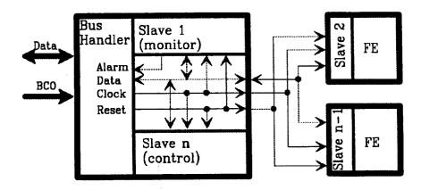
Figure 2 A schematic layout of the distributed CM circuit.
