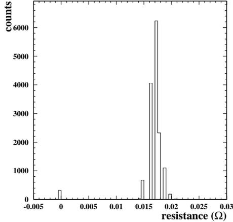
Figure 17: Histogram of resistance between ground shields on either end of the cable, taken from a sample of 575 vacuum cables. Those measurements which resulted in an open ( $\infty \Omega$ ) were recorded as  $0 \Omega$ .
