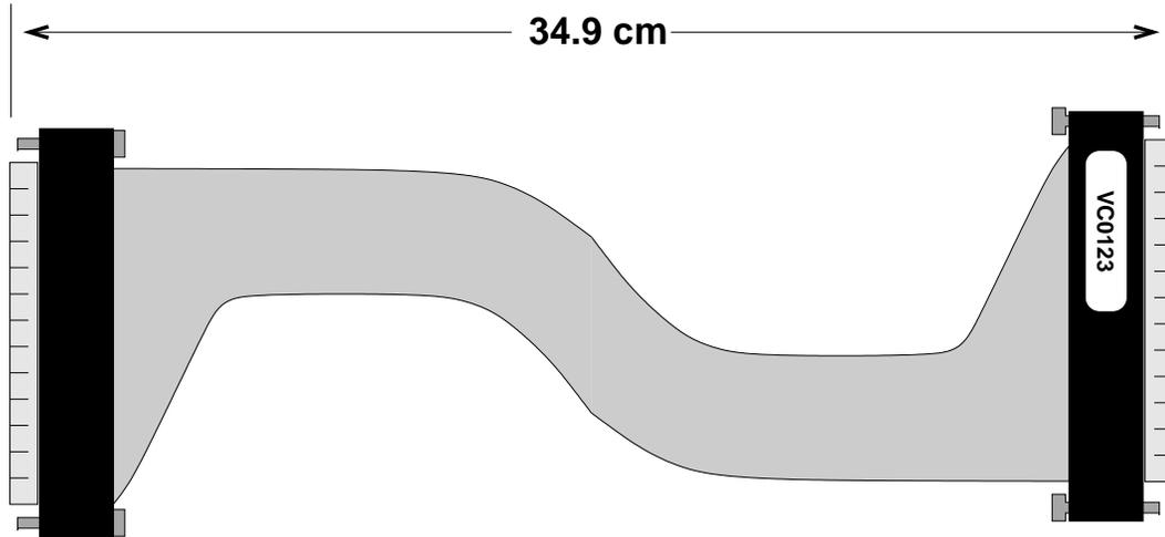
Figure 2: A schematic of an endcap feedthrough vacuum cable.
