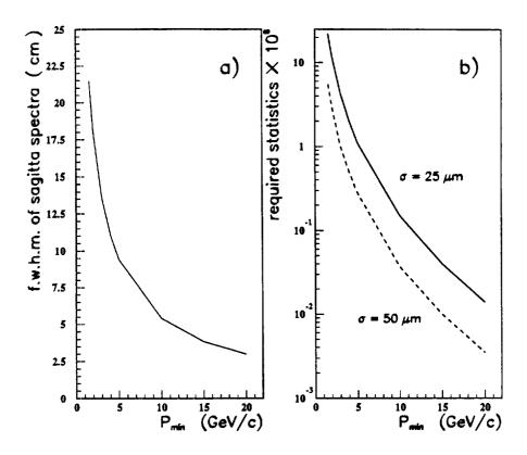
Figure 3: (a) - Dependence of the width of the sagitta spectrum on the low momentum threshold of registered particles; (b) - Statistics required to achieve an accuracy of 25  $\mu$ m (solid line) and 50  $\mu$ m (dashed line) for different lower momenta thresholds.
