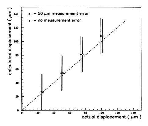
Figure 4: The correlation between actual and calculated displacement values for cases with and without coordinate resolution effects. A total of  $4 \cdot 10^6$  particles, with momenta greater than 3 GeV/c, are used for each point. The dashed line corresponds to a perfect correlation between actual and retrieved displacements.
