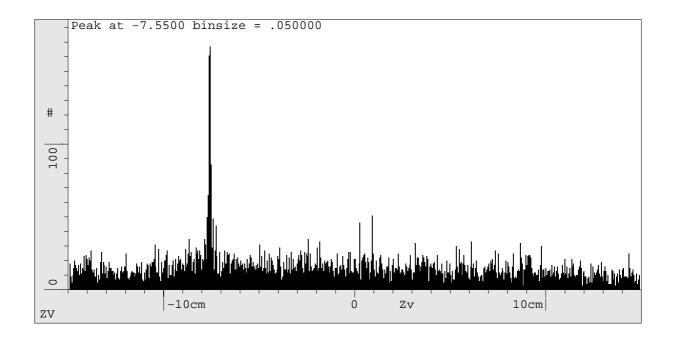
Figure 3: The z-histogram for the high luminosity/high- $p_T$  event using triplets of space points from the barrel Pixel and barrel SCT layers (22767 space points). The number of  $\phi$  slices was set to 1000.
