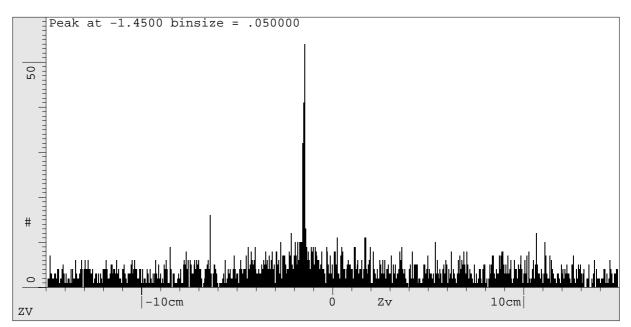
Figure 1: The z-histogram for the low luminosity/high noise/high- $p_T$  event using pairs of space points from the barrel Pixel layers only (2324 space points). The number of  $\phi$  slices was set to 1000.
