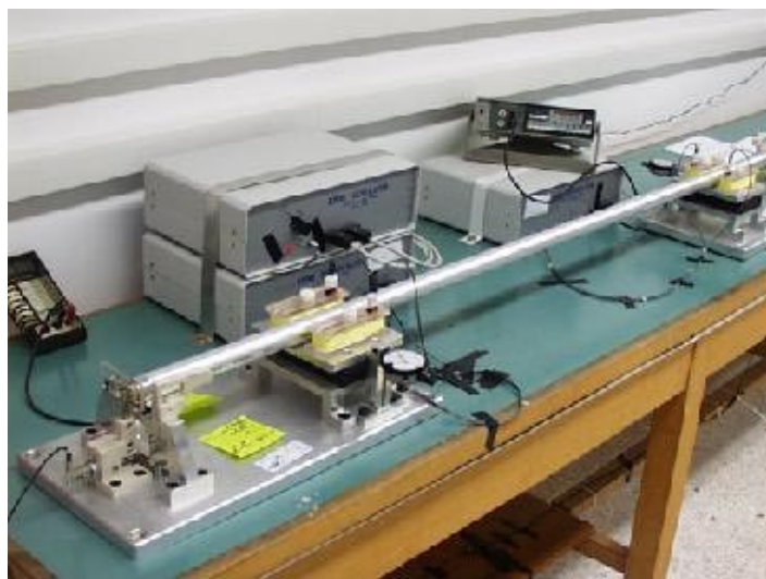
Figure 10: The EMMI system, the tube V-shape support and the coils.
