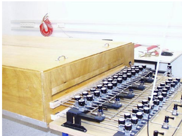
Figure 14 : Views of the thermally insulated box from inside and outside. Each vane is connected with the corresponding MDT detector in the box via a twisted narrower tube.
