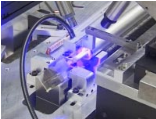
Fig. 3. Precise wire positioning using glue curing under UV illumination.
