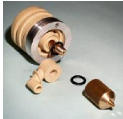
Fig. 4. Endplug design for the wire glueing technique.
