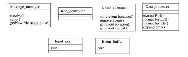
It is possible to describe the ROB Complex as an assembly of sub-systems which include the classes described above.
