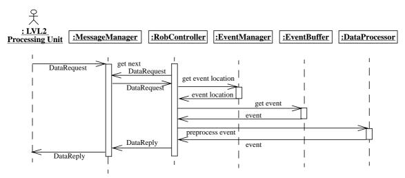
The presented scheme is not mandatory. Here, it is developed but it is possible to compress the path followed by data. In particular, in some cases, data location can be directly provided to the message manager instead of a copy of the event. In the Rob Controller, only the frame of the reply is built. In the same way, the data processor can access to the event buffer to get data to
