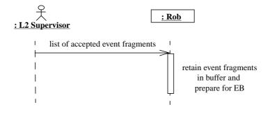
An other scenario based on an architecture similar to the LVL2 architecture has been proposed for event building. The L2 Accept is not directly sent to ROB but to EB. The later distributes to all ROBs the L2 Accept with the address of the farm which will process the event.
