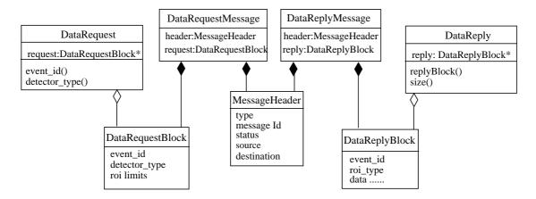
The actual request is the DataRequestBlock. To travel, it is dressed with the DataRequestMessage. A MessageHeader is added at top. When sited in a node of the system (Rob or Processing Unit) a DataRequest class gives access to the inside of the request.
