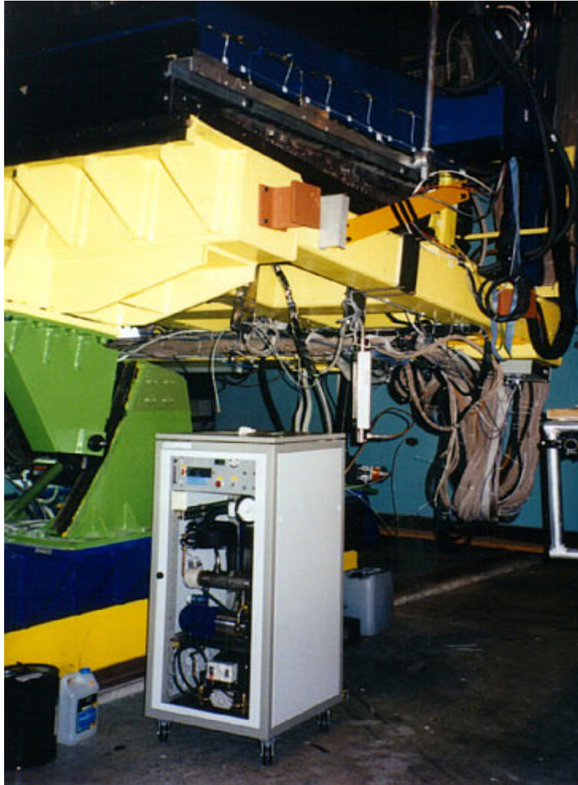
Figure 4: Photo showing the C_6F_{14} cooling rack below the TILECAL module.
