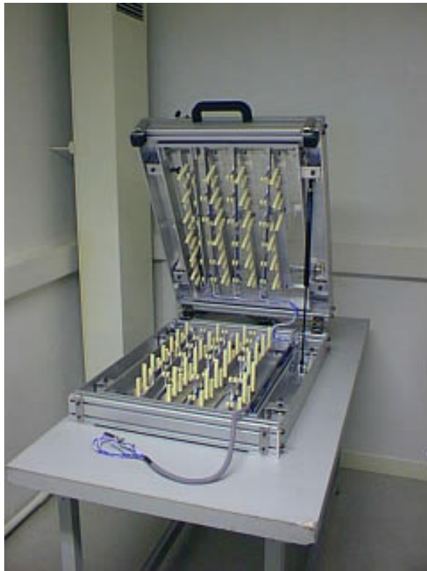
Figure 6: Bench for the bent electrodes C : Mechanical support keep the tested electrode in shape
