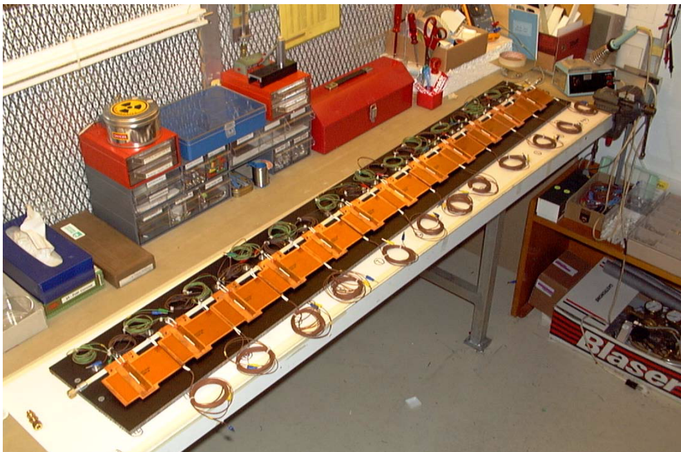
FIGURE 13. Full length prototype, fully equipped with one row of Cu-based thermal modules
