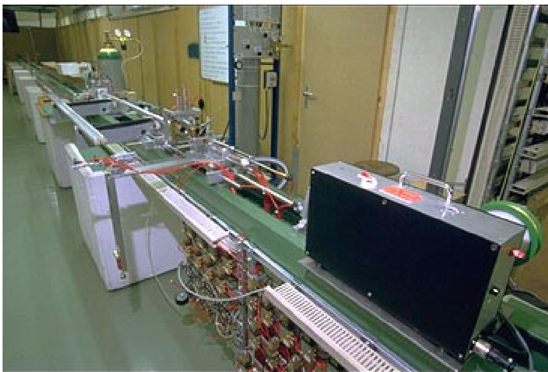
Figure 2: The test stand of the prototype wiring automate
