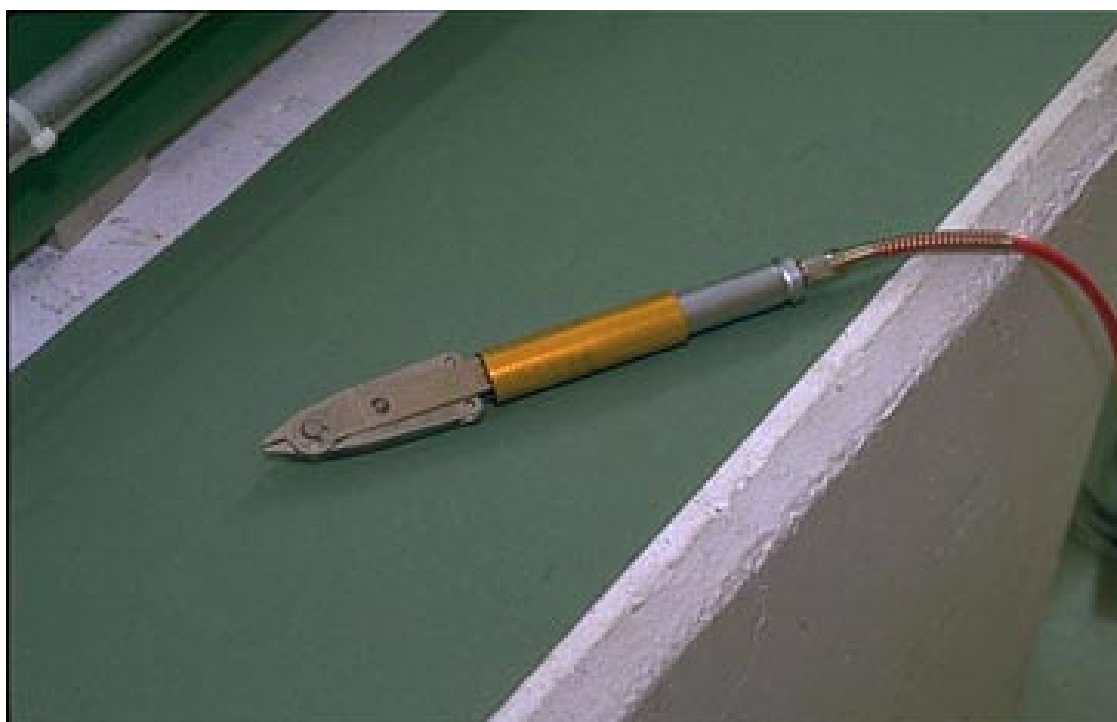
Figure 20: The pneumatic pair of pliers to crimp the wire, developed at CERN
