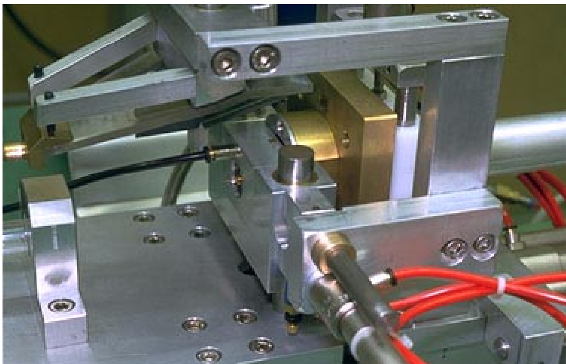
Figure 17: The far endplug is pushed into its final position to be pressure crimped in the aluminium tube
