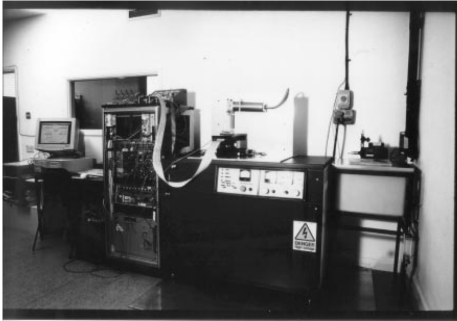
Figure 1: Photo of a general view. From left to right: PC, rack with DAQ electronics, X-ray scanning facility on top of the high voltage power supply.
