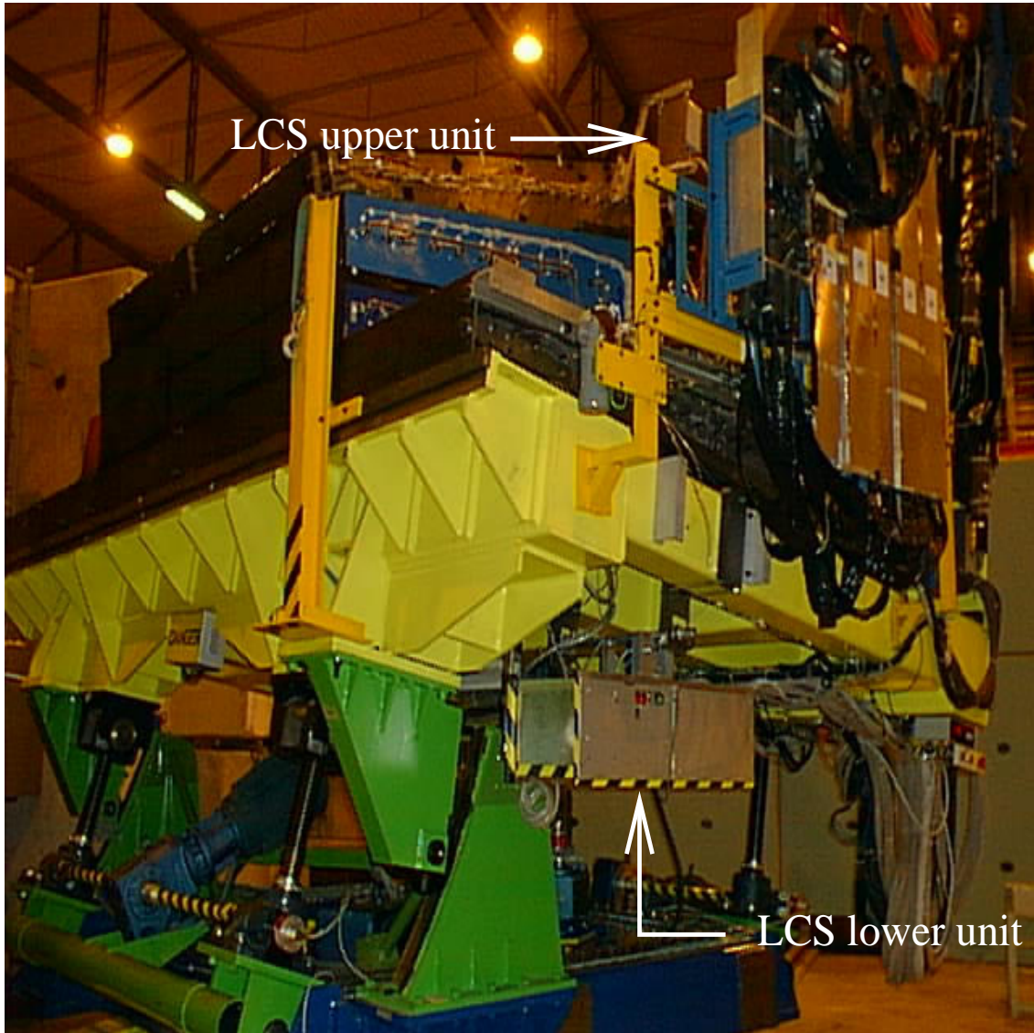
Figure 5: Photo of the test beam experiment with the lower unit of the cooling system just under the table and the upper unit above.
