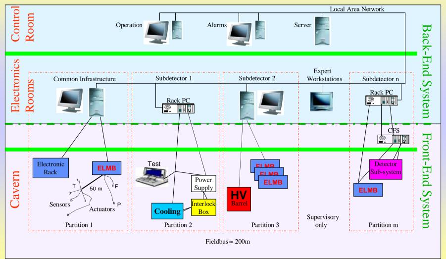
From sensors/actuator up to complex computer-based systems e.g. VME, PLC Specific and general purpose fieldbus I/O modules e.g Embedded Local Monitor Board
