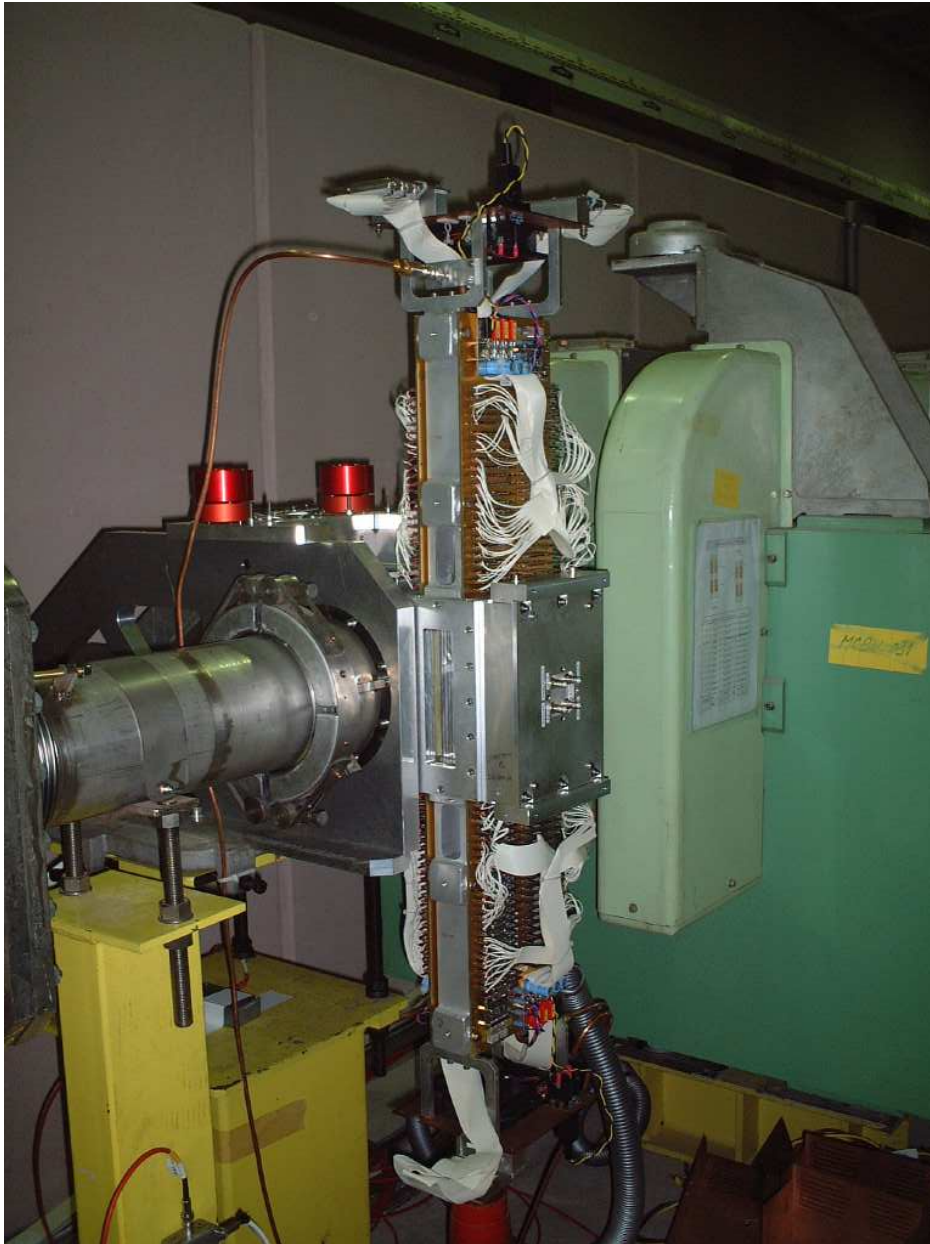
Fig. 17: The KABES-1/2 detector, which are moved horizontally by \sim 20 cm outside the beam line to show the entrance window.
