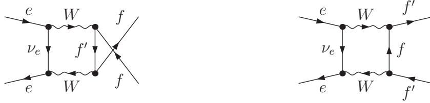
Figure 2: Electroweak W–W-box diagrams at the one-loop level, where f denotes an isospin-up and f' an isospin-down fermion.
