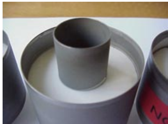
Figure 1: Ceramic disk brazed onto titanium conductors
