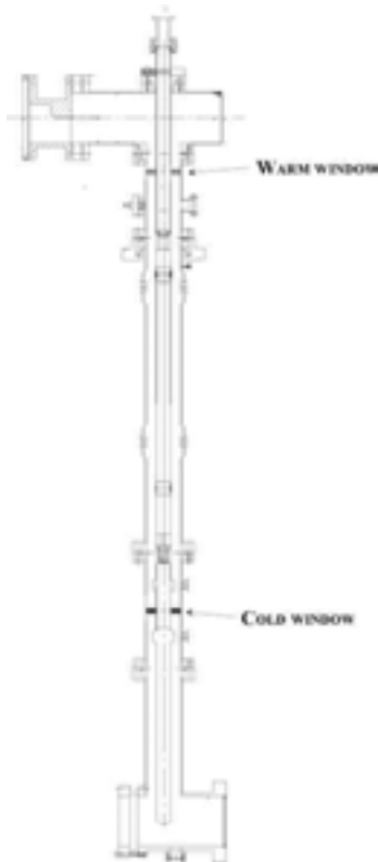
Figure 5. Schematic of the prototype coupler.
